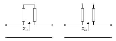
$\boldsymbol{Z}_{in}$  is the input impedance of the series circuit. The ABCD-parameters for the series stub are calculated as
