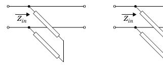
$\boldsymbol{Z}_{in}$  is the input impedance of the shunt circuit. The ABCD-parameters for the shunt stub are calculated as
