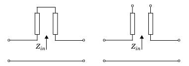
${\cal Z}_{in}$  is the input impedance of the series circuit. The ABCD-parameters for the series stub are calculated as
