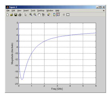
**7** Analyze the data object over a new frequency range. The original S-parameters are given over the frequency range 315KHz to 6GHz. If you want to see the S-parameters over a new frequency range, you need to analyze the data object first.
