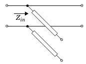
$\boldsymbol{Z}_{in}$  is the input impedance of the shunt circuit. The ABCD-parameters for the shunt stub are calculated as
