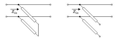
$\boldsymbol{Z}_{in}$  is the input impedance of the shunt circuit. The ABCD-parameters for the shunt stub are calculated as
