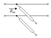
$\boldsymbol{Z}_{in}$  is the input impedance of the shunt circuit. The ABCD-parameters for the shunt stub are calculated as
