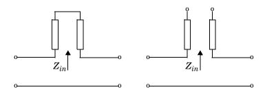
$\boldsymbol{Z}_{in}$  is the input impedance of the series circuit. The ABCD-parameters for the series stub are calculated as
